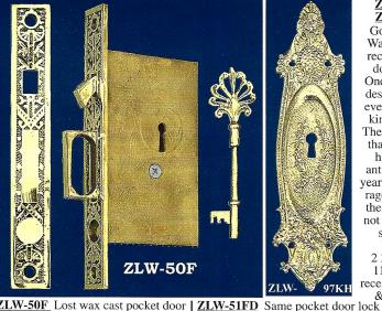
**ZLW-50F** Lost wax cast pocket door lock & catchplate, for a single pocket door. Lock Body: 5"h x 3"w by 1/2" thick case. 2" backset. Lockface size and catch plate size are: 7" h x 1" w
