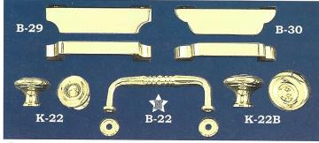
Contemporary solid brass hardware, All use 8/32" thread for mounting. B-22 Lathe turned/wrought bail w/ 19/32" dia lathe turned washers 3" boring B-29 Precision Cast concave ends brass handle with internal recess. B-30 Precision Cast convex ends brass handle with internal recess. Both B-29 & B-30 are 3/8" thick and meas: 3" w x 3/4" projection; 2 1/2" c/c
