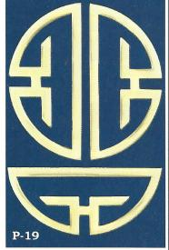
P-19 Heavy wrought brass Chinese design handle, or, when two are used--a center piece on two adjoining cabinet doors (separate 1/2" for 5" circle effect). Each Meas: 5" x 2 1/4"; mounts on 3 leg studs on the back of the handle w/ 8/32 machine screws. 3/16" material thickness.
