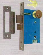
ZC-103SP Outside entry plate with ZC-104TL inside entry plate and L-9SPAC-DL Plates measure 21" h x 3 1/2" w. Lock body is 5 1/2" h x 3 5/8" w x 13/16" thick. Lock face is 1" w x 7 1/2" h with a 2 1/2" backset. This Vintage Hardware lock set makes an elegant and complete Arts & Crafts style entry for your door. All Pieces are made of solid copper and hand hammered including the strikeplate and lock face.
